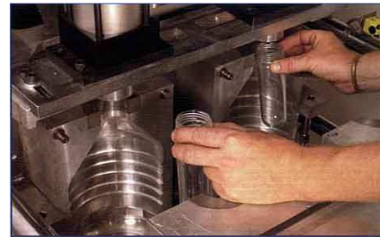
Fig. 4: Preforms, after being heated in the Preheater are transferred to the Blow Moulder
