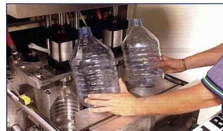
Fig. 5: Bottles after being formed are removed from the two-cavity mould.
